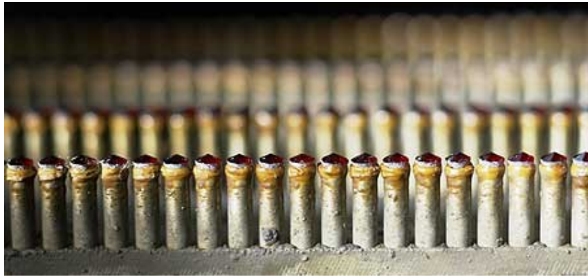
The prepared pyrope after machine grinding from one side before cementation.
